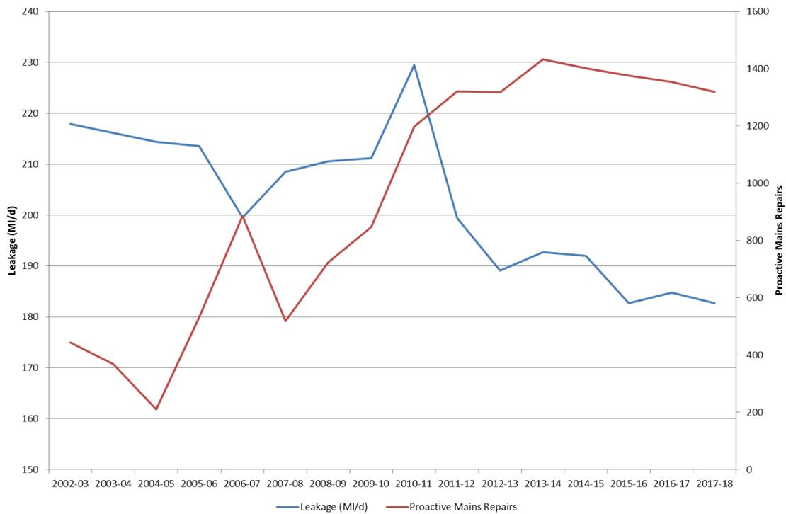
The graph above illustrates how proactively detected bursts relates to reduced leakage levels.
