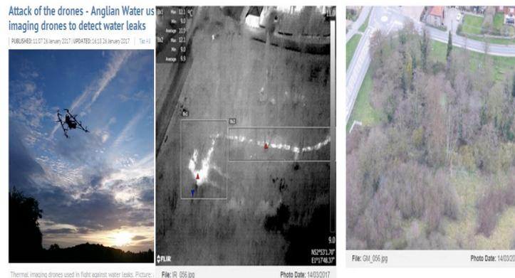
Thermal imaging drones used in fight against water leaks. Picture: File: IR\_056.jpg Photo Date: 14/03/2017
