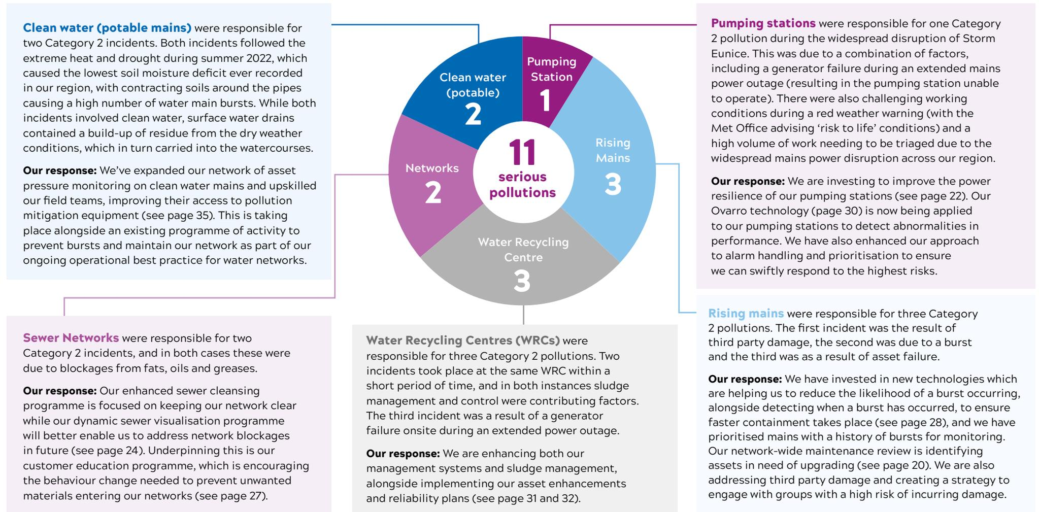
**Clean water (potable mains)** were responsible for two Category 2 incidents. Both incidents followed the extreme heat and drought during summer 2022, which caused the lowest soil moisture deficit ever recorded in our region, with contracting soils around the pipes causing a high number of water main bursts. While both incidents involved clean water, surface water drains contained a build-up of residue from the dry weather conditions, which in turn carried into the watercourses.
