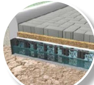
A CROSS-SECTION OF A CITY STREET PERMEABLE SURFACE
